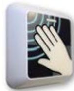
By using motion detectors or a ClearWave control, the staff does not need to touch anything to open the door quickly, which keeps their hands clean. The Ixio-D is a radar and motion detector in one. It opens the door and monitors the passage at the same time.
